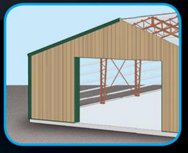
Attach pre-cut 40 year warranty sheet metal for walls and roof using supplied weather tight pre-painted fasteners.
