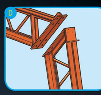
The roof truss easily connects to the sidewall leg, connecting with heavy duty plates and structural bolts.
