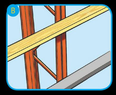
Wood or steel girts attach to the pre-welded clips with supplied fasteners every 2' giving superior strength and ease of interior finish.
