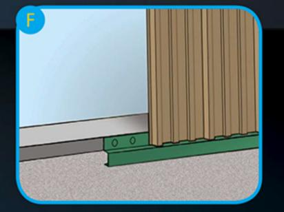
Attach the base trim to bottom girt to create a seal guard against the intrusion by rodents or insects.
