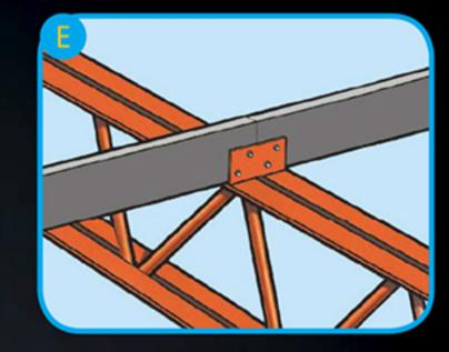
Wood or steel purlins set on top of the steel truss attached to pre-welded clips with supplied fasteners every 2'.
