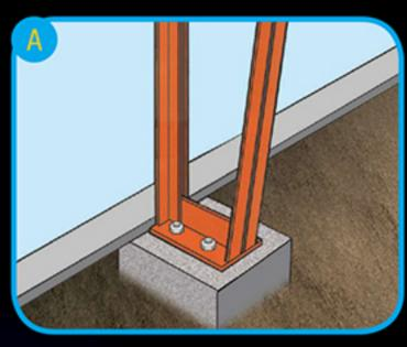
Setting the legs on full floor or basic concrete piers anchors building securely.
